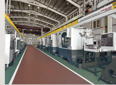
Aluminum Wheel Production Equipment
